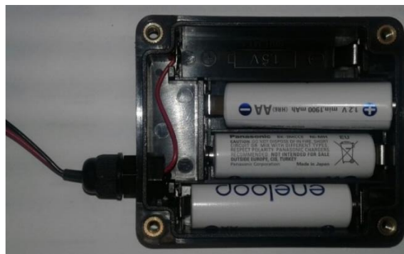
Fig. 18 – Replacing battery in battery box
